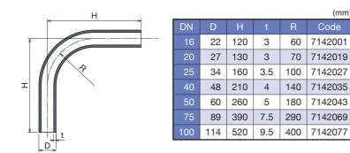
(Note) As the pipe is bent by softening the material with heat, the degree may change when the ambient temperature rises. Store the products in a well-ven tilated area while avoiding direct sunlight.
