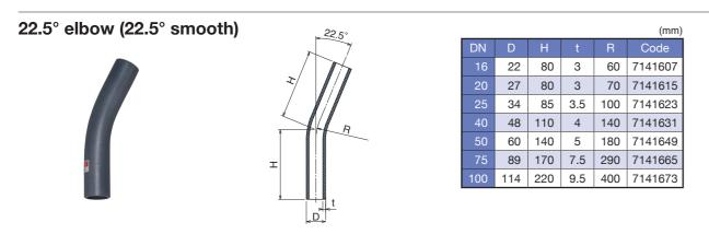
(Note) As the pipe is bent by softening the material with heat, the degree may change when the ambient temperature rises. Store the products in a well-ventilated area while avoiding direct sunlight.
