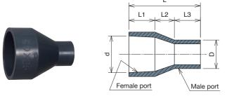
(Note) 1. As a drawing process has been performed on the product of the size marked with an asterisk (\*) by softening the material with heat, the diameter may change when the ambient temperature rises. Store the products in a well-ventilated area while avoiding direct sunlight. 2. It cannot be used for electrofusion joining.
