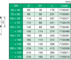
(Note) For joining, EFS, EFL, and EF-45 are needed
