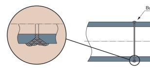
\*The operation of only butt joining of pipes is not performed in principle. This construction method is performed only when it is necessary.
