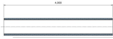
GRP pipe (glass reinforced polypropylene double-layer pipe)
